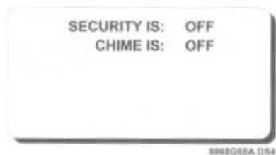
Figure 24. Status Display after Canceling a Panic Alarm
